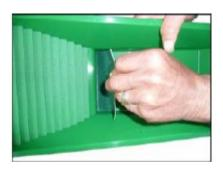
3. Gently lay the remainder of the grit strip down assuring proper alignment with the sides before pressing all parts of the grit strip down firmly.
